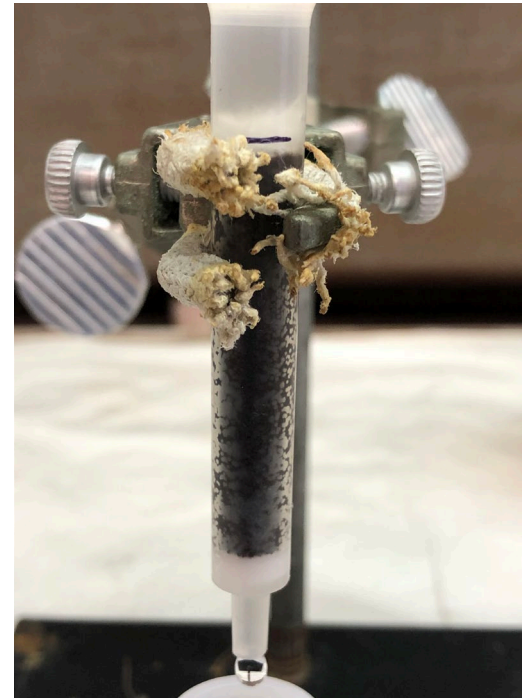
Gas production restricting flow rate under gravity
