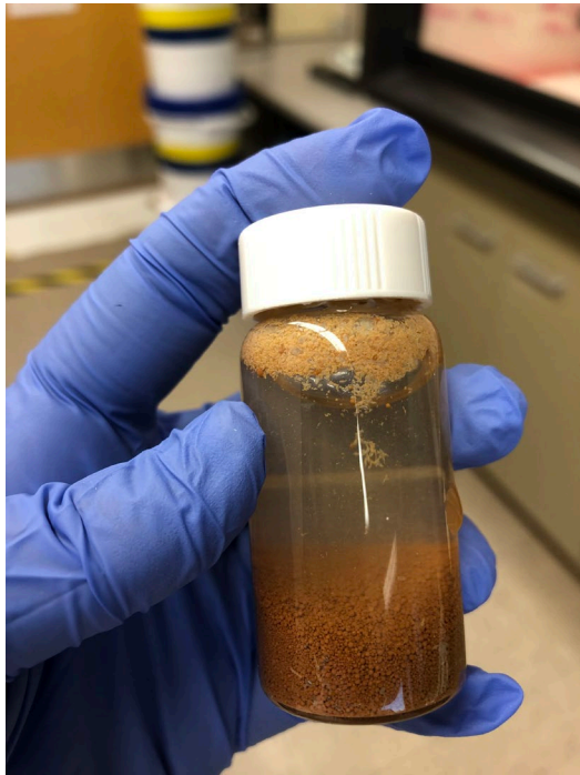
Small floaters had to be decanted when prepping slurry to prevent column clogging
