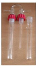
HTO / H<sub>2</sub>O trapped from exhaust gas
