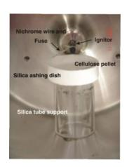
Sample loaded into disposable silica crucible
