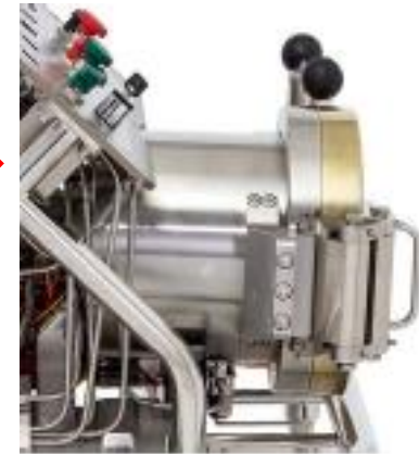
Improved pressure vessel with resistance wire ignition
